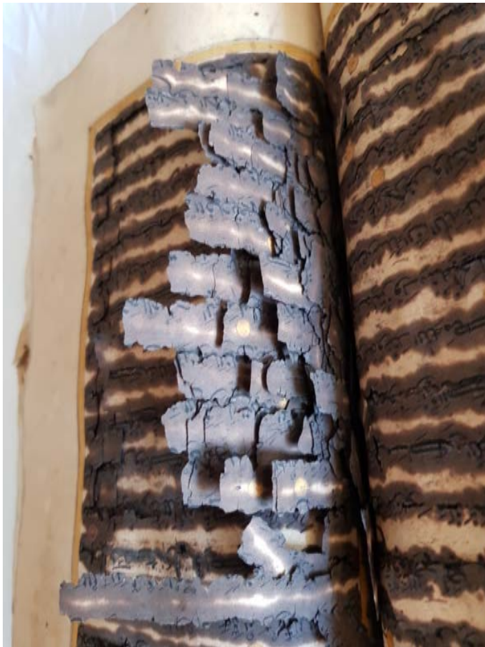
Damage to the paper pages caused by the corrosion of the iron gal ink. Image courtesy of the Pahang Museum and Alex Teoh
