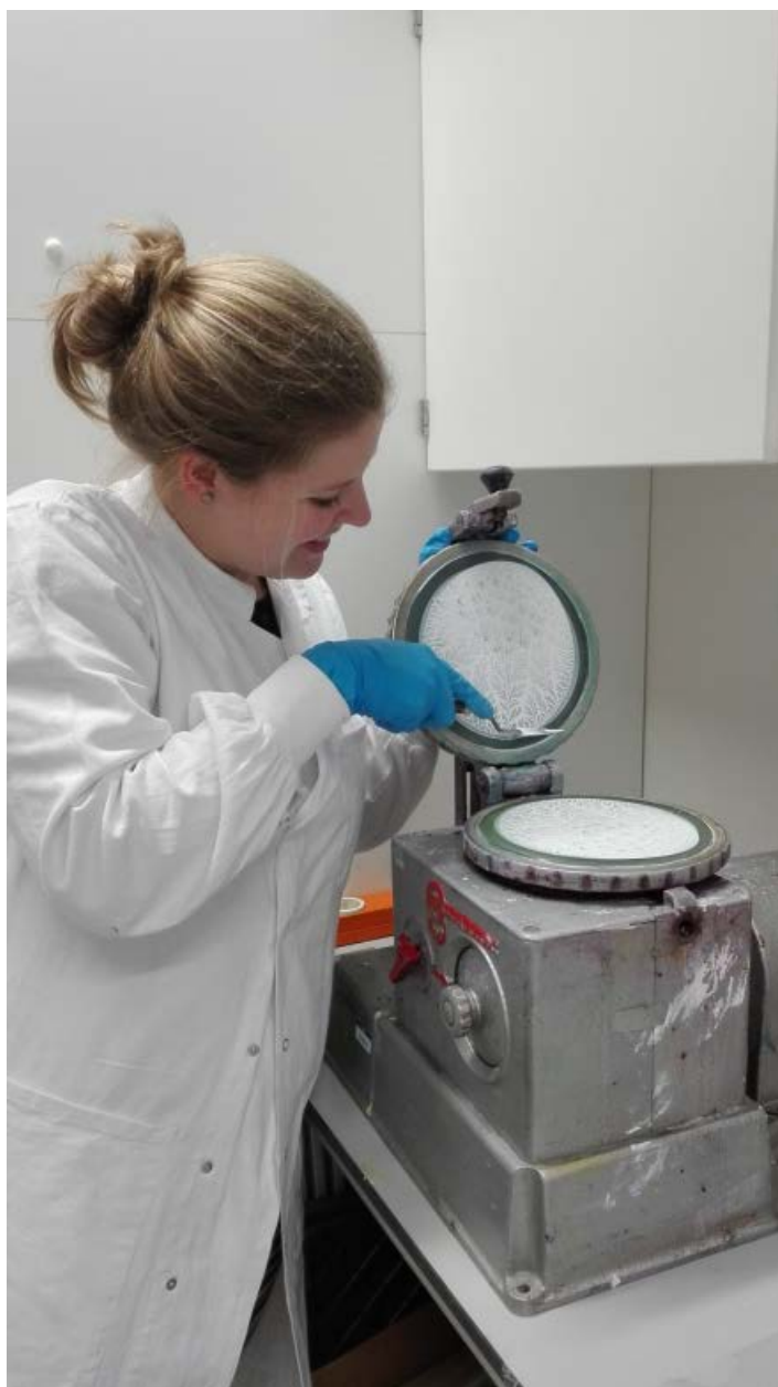
van Driel preparing titanium white oil paint samples on a glass-plated mill in the lab of the Cultural Heritage Agency of the Netherlands (image provided by the author)
