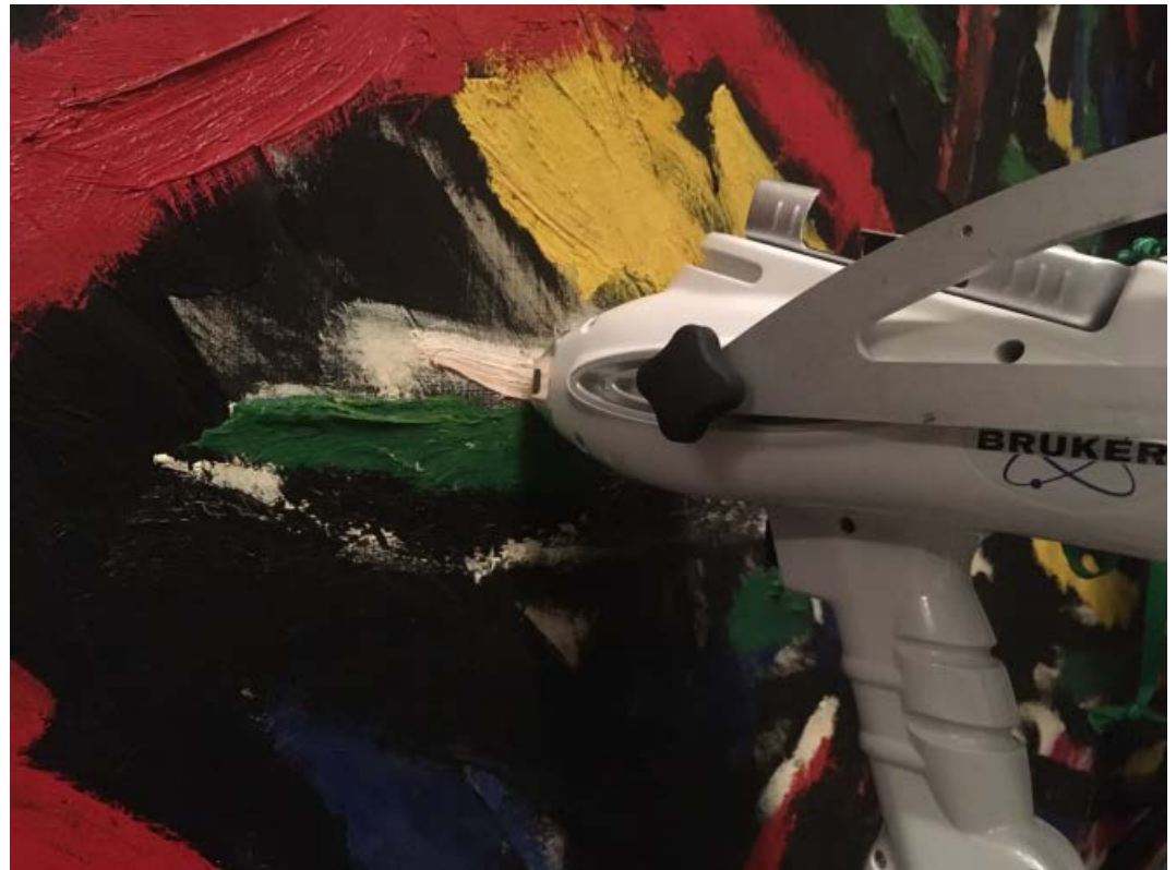
XRF analysis on a white paint stroke using a Bruker III-SD (Image provided by the author).
