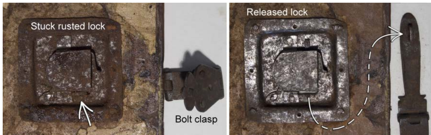
Inner back cover, after removing the pastedown. Right: The bolt clasp is still stuck into the lock and both pieces are visibly rusted. Left: Unlocked lock and bolt clasp, after removing rust. © Rita Udina
