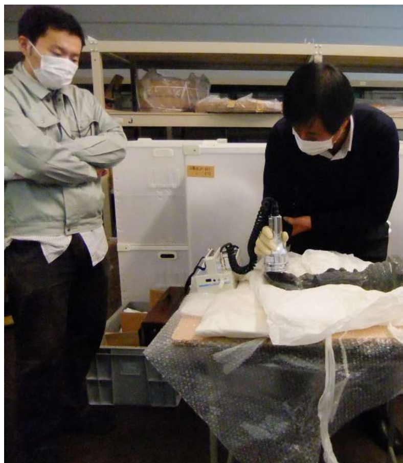
Top left: Measurement of radiation contamination of cultural properties at a temporary storehouse after rescue.
