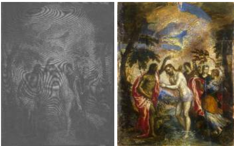
The fringes visualise the effect on the surface of detachment
